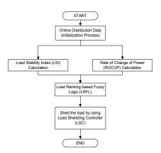
Figure 1. Overall concept of adaptive UFLS
